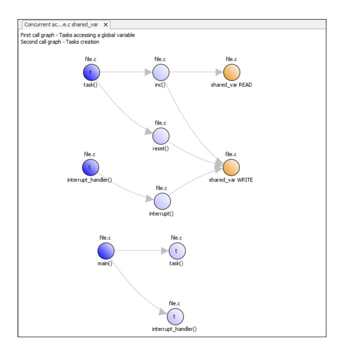
The first graph shows how the tasks access the variable. For instance, the task interrupt\_handler calls a function interrupt that writes to the shared variable shared\_var.
